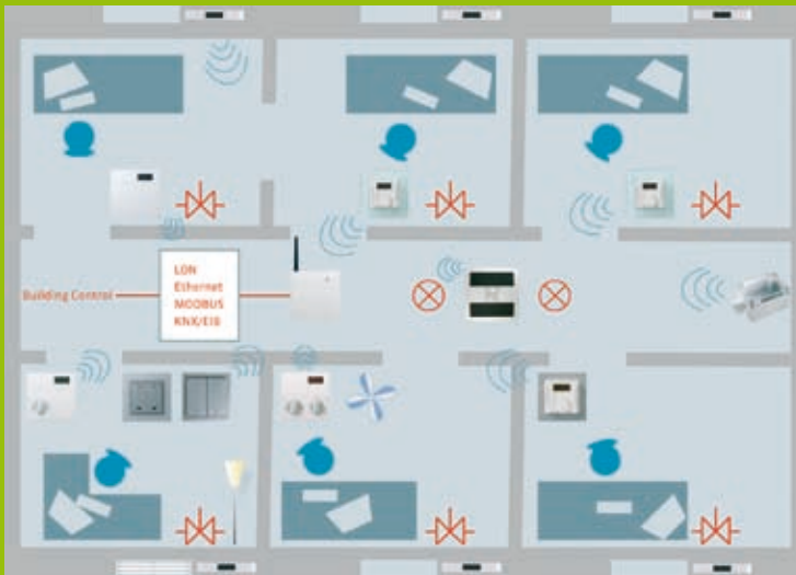
Floor plan illustrating use of EasySens in building
