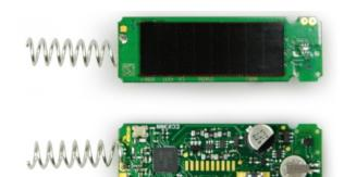
Power is provided to STM 350U by means of a small pre-installed solar cell which works in conjunction with an integrated energy storage element in order to ensure operation in periods without ambient light.
