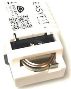
Figure: Properly inserted battery
