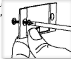
C. Insert the first screw loosely and level the module.
