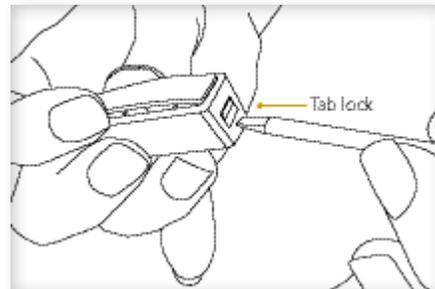
The cover is removed from the magnet body.
