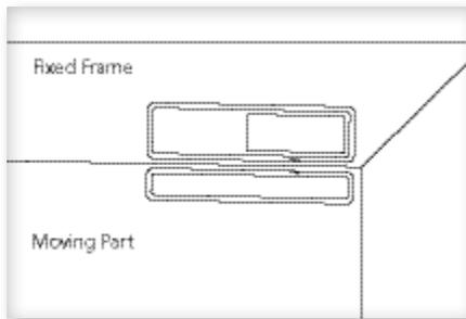
NOTE: For low activity applications, the magnet can be mounted with double-sided tape (not included).
