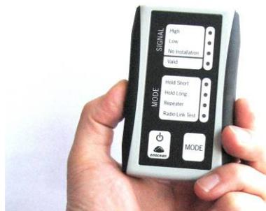
Figure: Field intensity meter EPM 300
