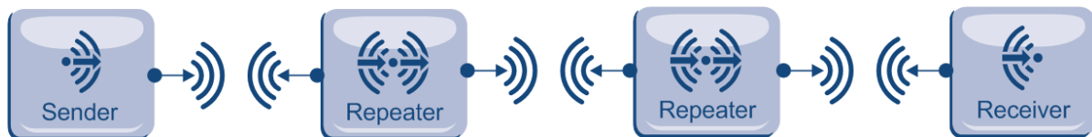
Figure 2 Range extension through repeaters
