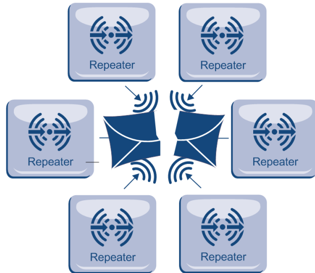
Figure 3 Not allowed repeater configuration
