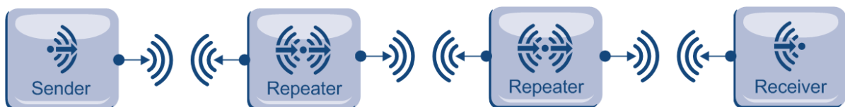
Figure 2: Range extension through repeaters
