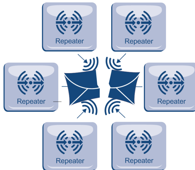
Figure 3: Not allowed repeater configuration
