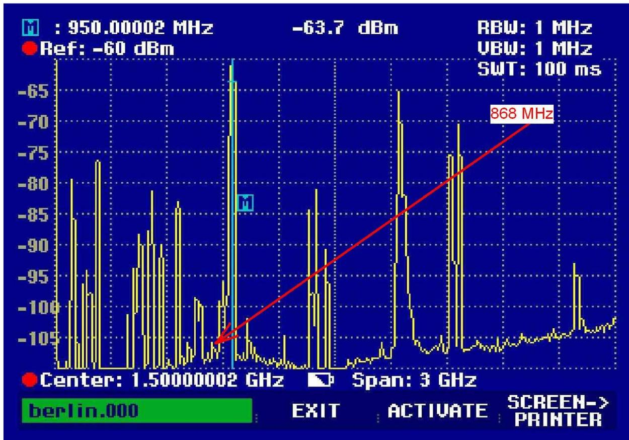
Fig. 3: A Very strong jammer sample was recorded near a wide band power radio transmitter with directive antenna. It is very clear to see here that there are the high levels around the 150, 600, 950, 1400, 1900, 2200 MHz frequency range.
