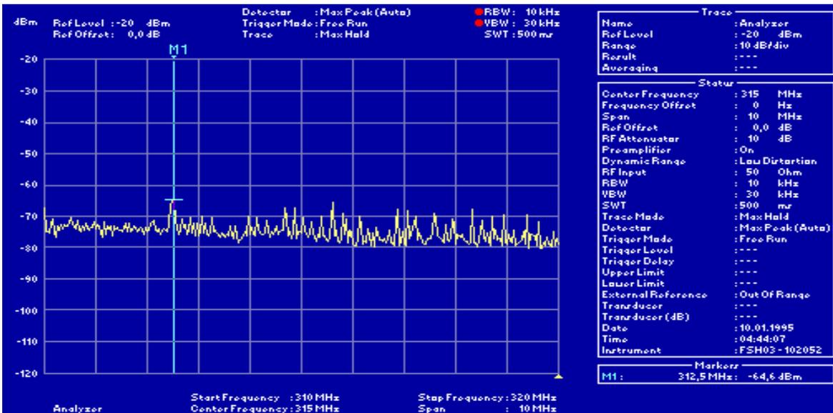
Fig. 2: Same with external preamplifier. Please note the higher floor level due to the additional external preamplifier (preamplifier gain: +37 dB)
