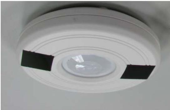
Fig. 1: Light powered Motion Sensor (Prototype)
