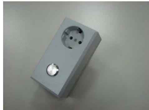
Fig. 2: Line Powered Wall Receiver (Prototype)
