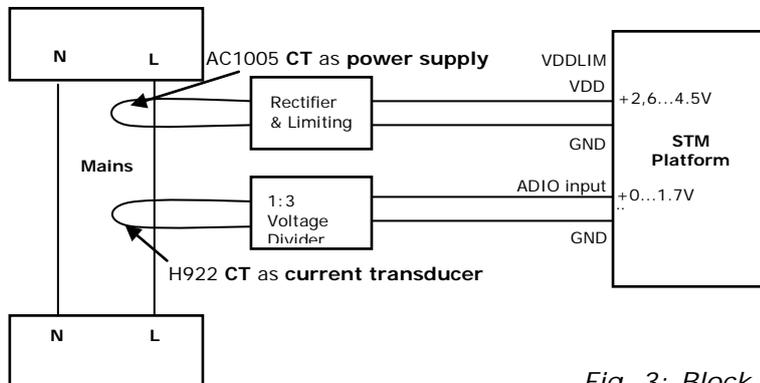
Fig. 3: Block Diagram of the Current Sensor
