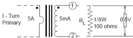
Fig. 4: CT Equivalent Schematic
