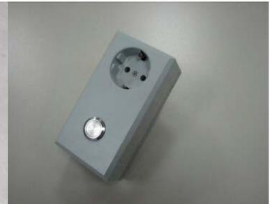
Fig. 3: Line powered TCM based radio controller
