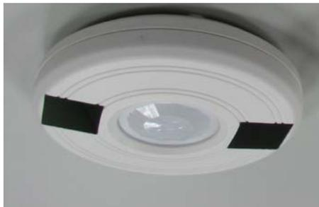
Fig. 1: Ambient light powered Motion Sensor
