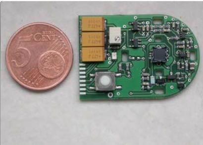
Fig. 2: STM based Motion sensor (front view)
