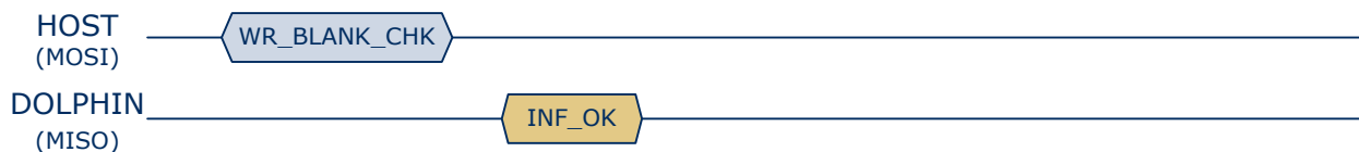
Figure 21 – Command WR_BLANK_CHK (erased state)
