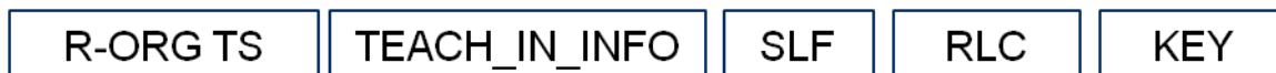
Figure 13 Secure teach-in message. Teach-in Info field contains information relative to the teach-in message itself. The SLF field indicates the format of the security parameters in operation mode. The RLC is the current RLC in the transmitter. The KEY contains the private key used for encryption in operation mode. RLC and KEY may be encrypted with a pre-shared key
