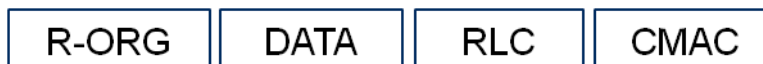
Figure 7. Relevant message members. In what follows the DATA member includes the DATA and OPTIONAL DATA.
