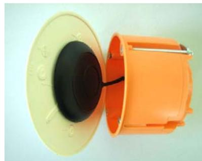
Figure: Mounting a Patch Antenna
