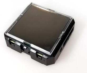
The solar-powered [STM 33x \(868 / 902 / 928 MHz\)](#) sensor, for example, can measure temperature in a room or on machinery. This module is characterized by its extremely low-power consumption and high reliability. If a measured value is transmitted every 15 minutes, for instance, 3.6 hours of charging in daytime of at least 200 Lux are adequate for continuous operation. With its energy storage mechanism fully charged, the module is functional for several days in complete darkness.
