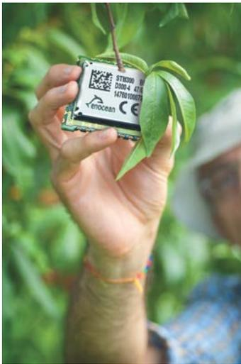
Energy can be found everywhere – in the movement of doors and windows or machine components, the vibration of motors, changes in temperature or variances in luminance level. These energy sources, which usually remain unused, can be tapped into by means of energy harvesting to power electronic devices and transmit wireless signals. This principle is the basis of energy harvesting wireless technology from EnOcean.
