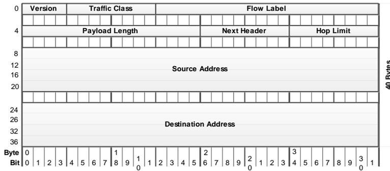
The IPv6 header structure
