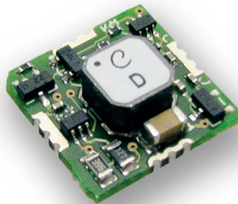
Fig. 1: ECT 310 DC/DC converter - works on as little as 20 mV, corresponding to 2°K temperature difference
