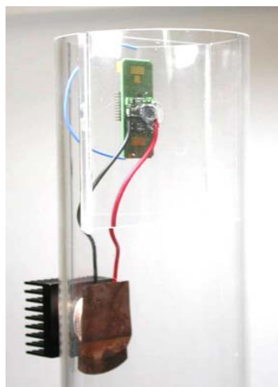
Fig. 3: Energy-autonomous sensor for air flow temperature
