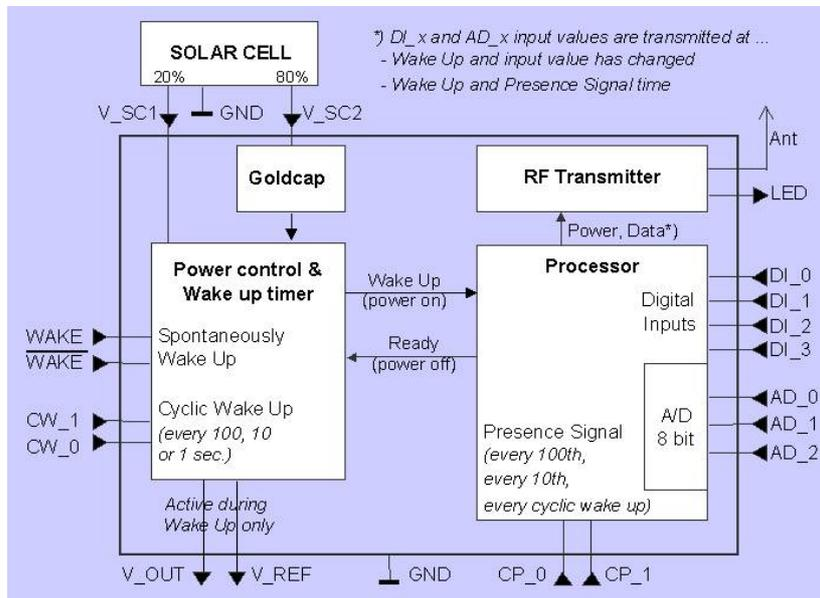
Figure 2: Block diagram showing the STM 110 radio sensor module
