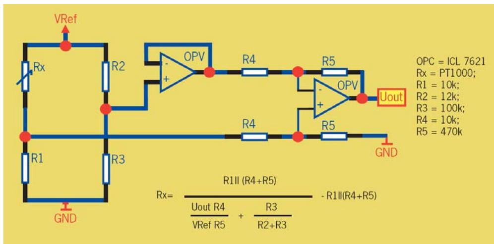
Figure 2: Additional external circuitry for implementing a solar-powered temperature sensor
