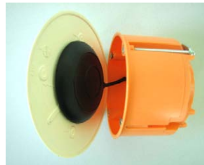
Figure: Mounting a Patch Antenna
