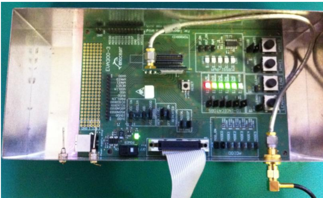
Figure 2. Example Gateway device in RF shielded enclosure with external antenna connector
