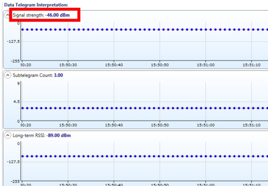
Figure 11 Operation with no attenuation, all sub-telegrams received
