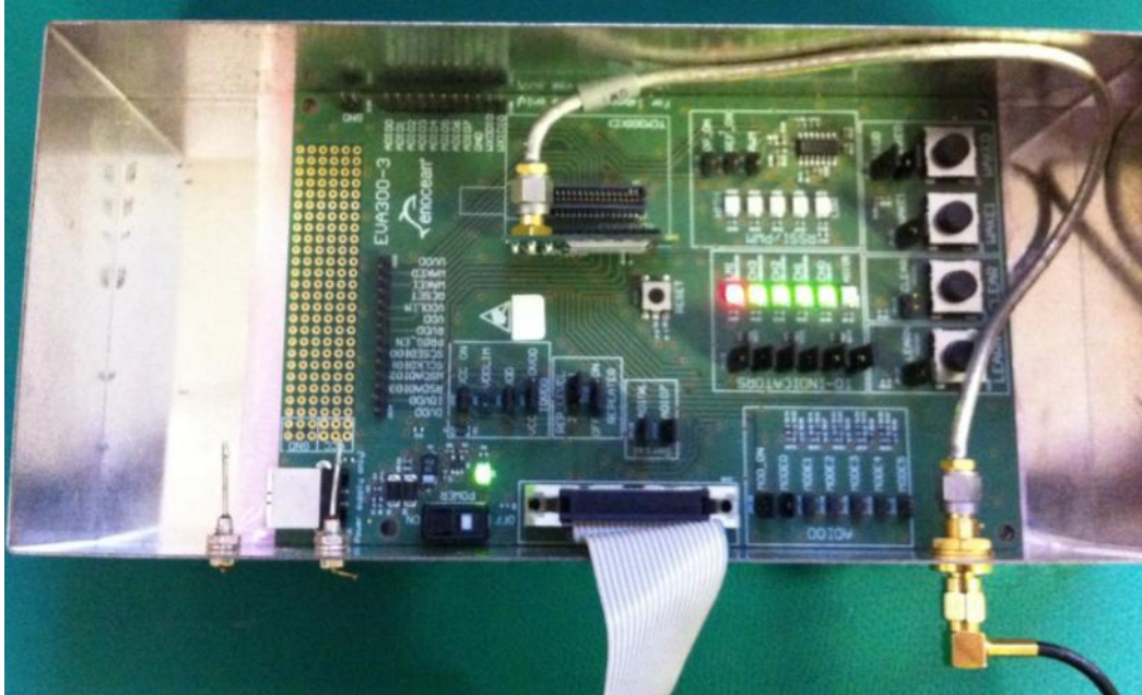
Figure 2 Example gateway in an RF-isolation enclosure with external antenna connector
