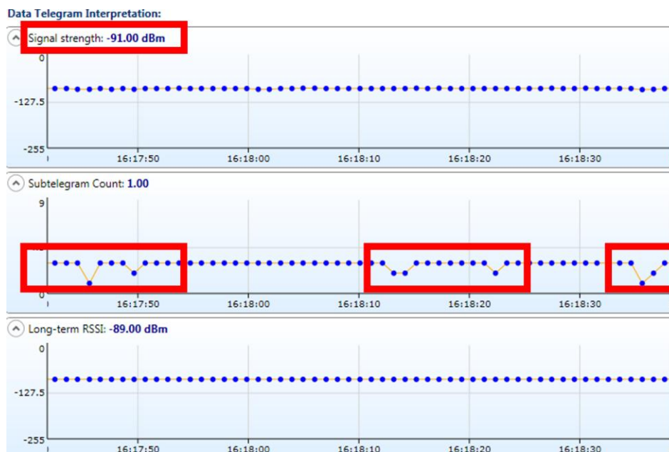
Figure 12 Operation at RX Sensitivity level
