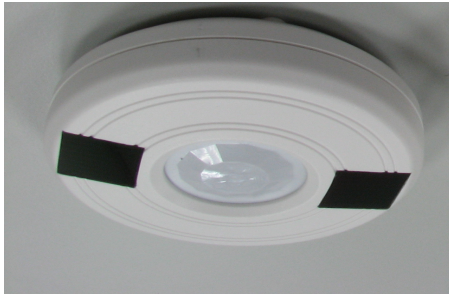
Fig. 1: Ambient light powered Motion Sensor
