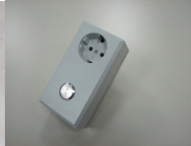
Fig. 3: Line powered radio controller
