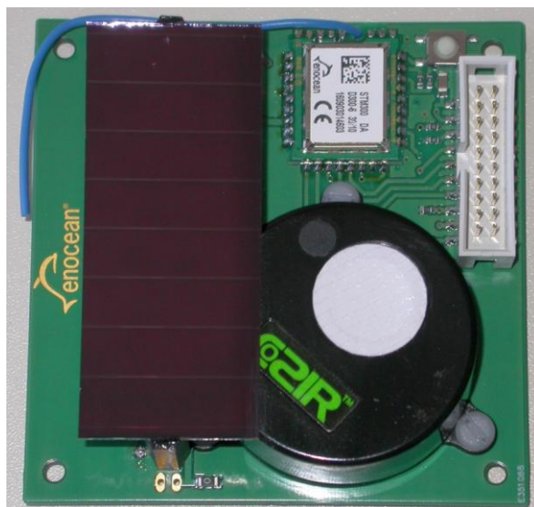
Figure 2 Solar-powered CO 2 sensor
