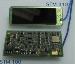
Due to the much higher level of integration the back side of the module could be emptied completely making room for a solar cell directly mounted onto the module.
