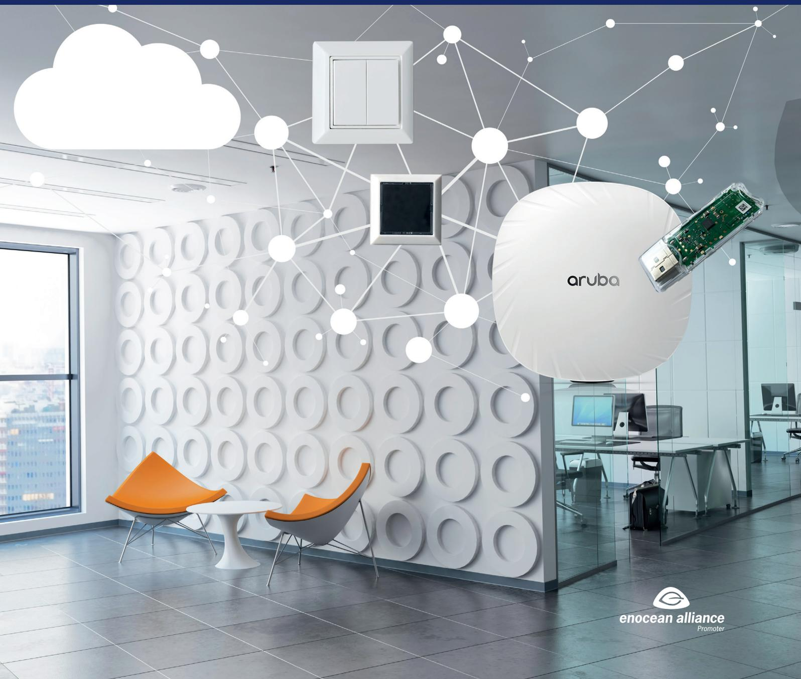
EnOcean and Aruba ensure a safe and cost-effective delivery of the collected data to the cloud for IoT projects in the building environment. The wireless, self-powered EnOcean sensors send the raw data via an EnOcean USB gateway to Aruba's Wi-Fi® access point, which pushes the data into the cloud. Companies can simply use their existing IT stick infrastructure and integrate IoT sensors into their network via Wi-Fi, in compliance with all security standards, thanks to Aruba.
