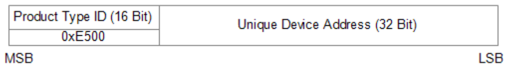
Figure 25 – BLE static source address structure
