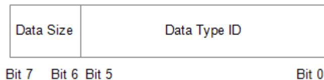
Figure 22 – Sensor Data Descriptor field structure
