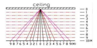
To provide coverage for very high ceilings, a wall sensor can be incorporated in the plan for complete coverage.
