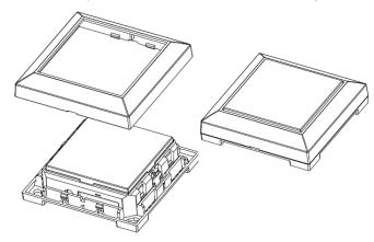
12. Should disassembly be required at a later point, insert a small flat screwdriver into the slot of the face plate (marked in green below) and push it upwards to remove it from the wall mount plate.
