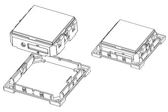
Note that backup battery and LRN button are protected from access after module installation into wall mount.
