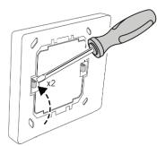
If necessary, the module can also be extracted from the front side without removing the wall mount from its installation location. To do so, carefully insert the screwdriver from the front between snap hook and module, press the hook outwards and lift out the module.
