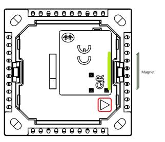
Attach the magnet to the intended surface (e.g. door or window) so that it aligns with the center of this side and verify that the distance between magnet and sensor housing is less than 1 cm (0.4 ").
