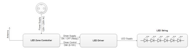
EnOcean LED zone controllers receive wireless input in the form of EnOcean wireless radio telegrams.
