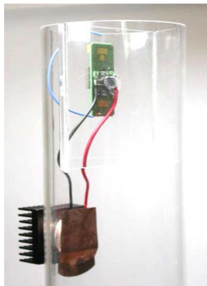
Fig. 3: Energy-autonomous sensor for air flow temperature
