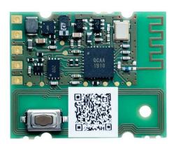
PTM 535Z transmits the status of the input signals and the action (press or release) of the connected ECO 200 kinetic energy harvester using the ON / OFF Switch model defined by the Zigbee Green Power standard.
