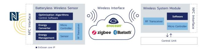
The NFC basic functions allow several different settings of NFC-integrating EnOcean modules. Therefore, self-powered switch and sensor modules with an NFC interface can be put into operation and commissioned very easily – even in the packaging – using NFC readers or NFC-enabled smart phones and tablets. The capabilities include:
